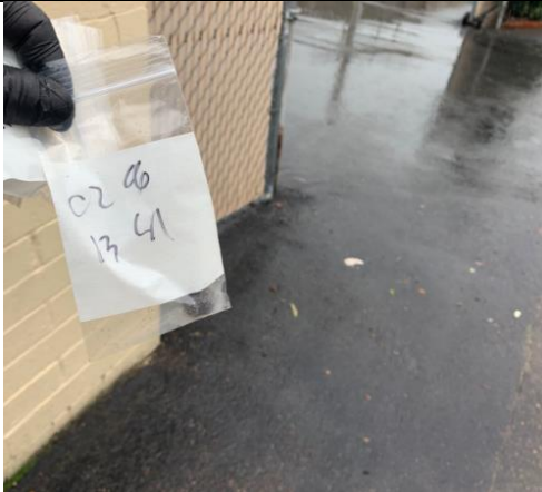
Photo of HA number 13, Sample No. 0206-13-41 | Non-ACM Black Asphalt, Within Parking Lot Station 18
