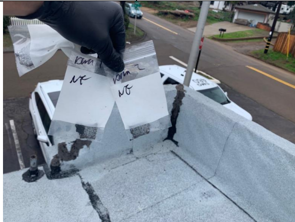
Photo of HA number 2, Sample No. 0206-02-05 0206-02-06 | Non-ACM Gray Parapet Wall, within Station 18 Roof
