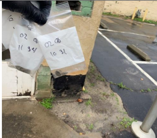
Photo of HA number 10 & 11, Sample No. 0206-10-31 & 0206-11-34 | Non-ACM Gray Block Wall & Gray Block Wall Mortar, within Exterior Station 18
